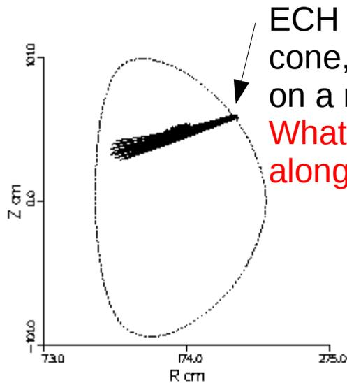
ECH injected in narrow cone, heats localized spot on a range of flux surfaces.
